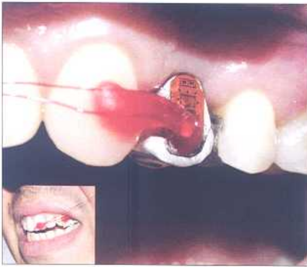
Figure 2. The solo contact at palatal cusp of partial crown provided the bending of strain gauge surface on the suprastructure. Intraoral position of experimental suprastructure during gum chewing.
