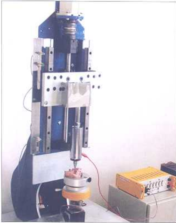
Figure 4. Functional load simulator and test model support with a load cell to gain feedback data to PLC.
